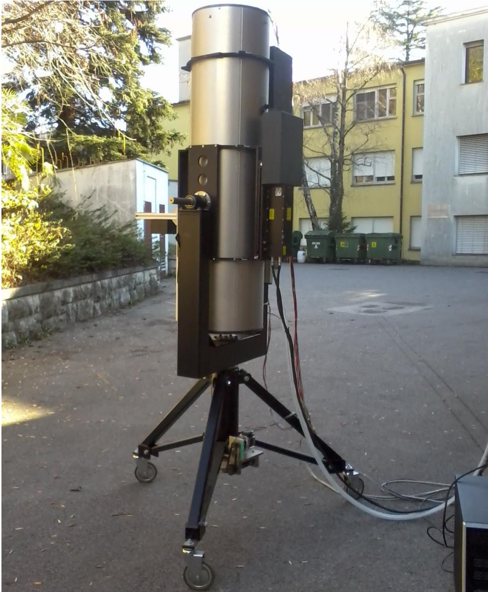
Figure 12: Working condition of the lidar system for vertical measurements at University of Nova Gorica on 14 January 2012. Data was taken in 5 minutes intervals from 06:00 to 22:00 CET. Solid state Nd:YAG (Quantel Big Sky) laser was used, operating at 1064 nm wavelength, providing 40 mJ pulse energy and 8 ns pulse width with repetition rate 10 Hz. Backscattered light was collected by the Newtonian telescope with a diameter of 302 mm. The signal was detected by EG&G C30954/5E Avalanche photodiode (APD) and digitized using TR40-160 Licel transient recorder with 12-bit resolution at 40 MHz sampling rate. Digital data was retrieved through an Ethernet link and stored on a Linux based DAQ computer.
