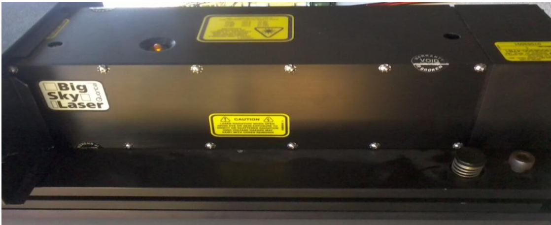
Figure 7: Quantel Big Sky laser used in the experiment. Top photograph shows its front panel with controls for pulse energy and frequency and the bottom photograph the laser head.
