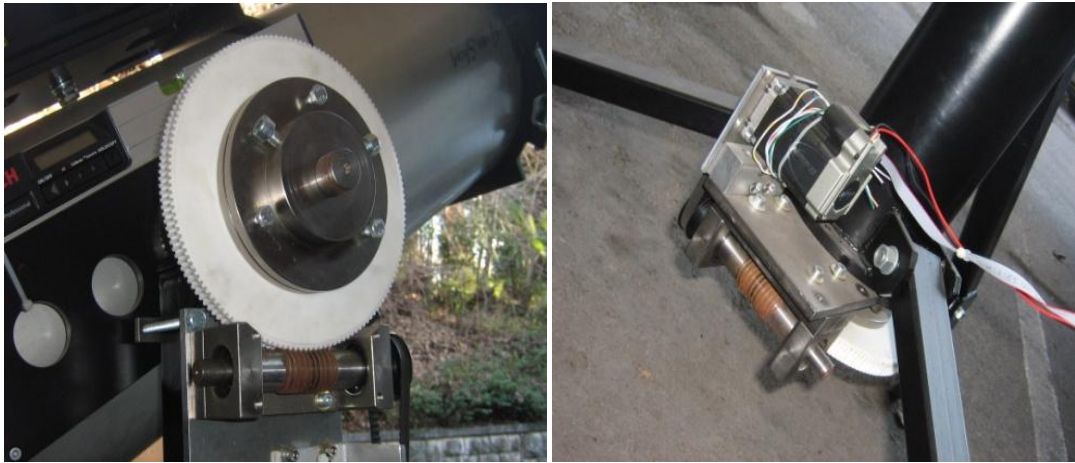
Figure 5: Servo motors and transmission systems for movement lidar. Azimuth and elevation angles can be set with 0.1^\circ precision.
