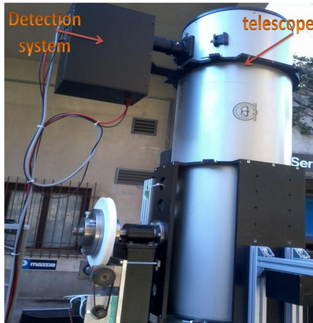
Figure 9: Detection system of the lidar. Return signals are detected by the photomultiplier tubes (PMT) for 266 nm and 295 nm channels and Avalanche photodiode (APD) for the 1064 nm channel. Receiver of the backscattered light is Newtonian telescope.
