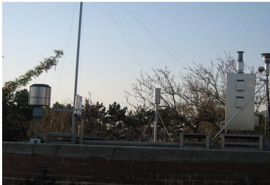
Figure 18: Air quality monitoring station by Slovenian Environment Agency located in Nova Gorica. The station continuously monitors wind speed and direction, temperature, relative humidity, air pressure, concentration of particles with size 10\mu m ( PM_{10} ) and NO_x gases.
