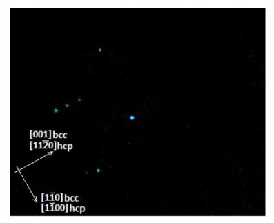
**Fig. 4.2** LEED pattern after 4 min of total Co deposition. Arrows indicate [001]bcc of Mo and [11-20]hcp of Co in one direction and [1-10]bcc of Mo and [1-100]hcp of Co in other direction. E=143.5eV
