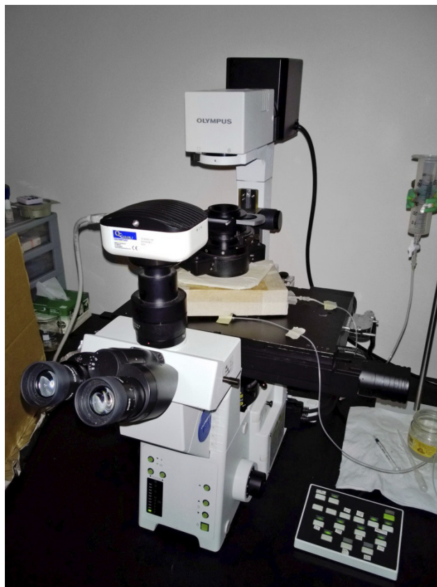
Figure 10: Epifluorescence microscopic setup ready for imaging
