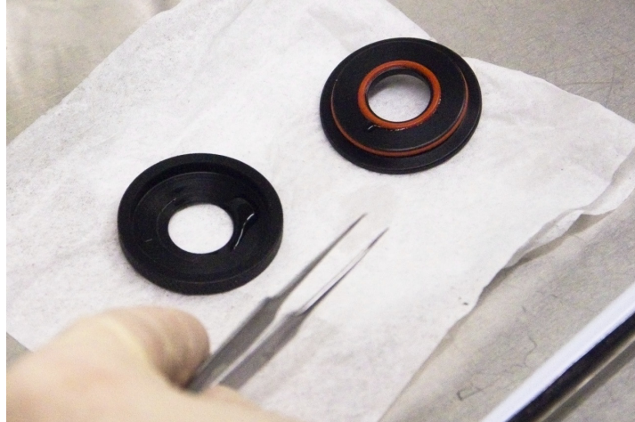
Figure 11: Insertion of the sample into the imaging chamber (imaging chamber disassembled)
