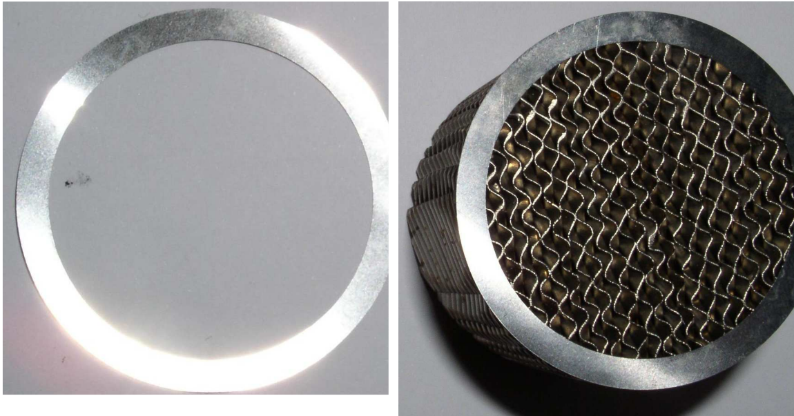
Figure 17: Ring made from stainless steel (left) and the same ring on the top of OCFS packing like in experiments (right)
