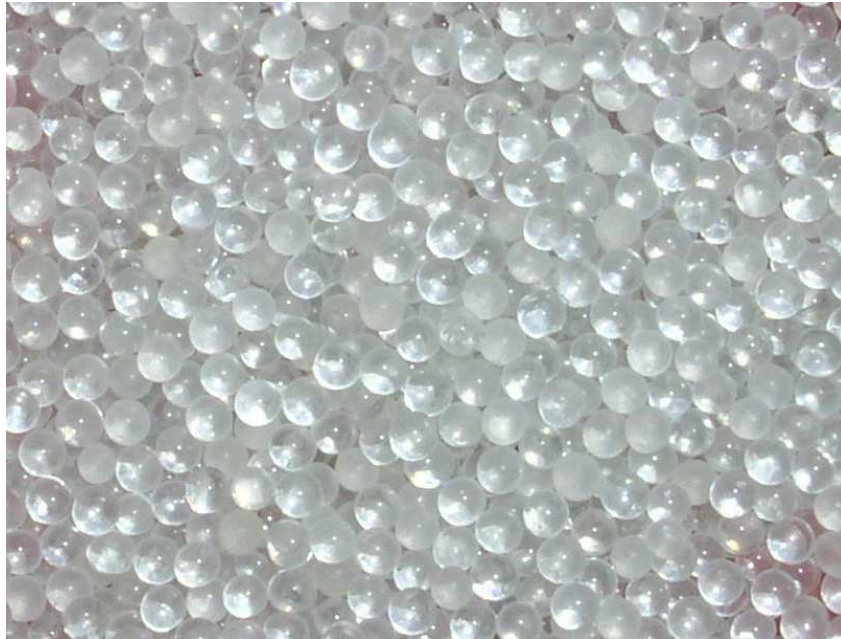
Figure 14: Glass bead used which are representing randomly packed bed
