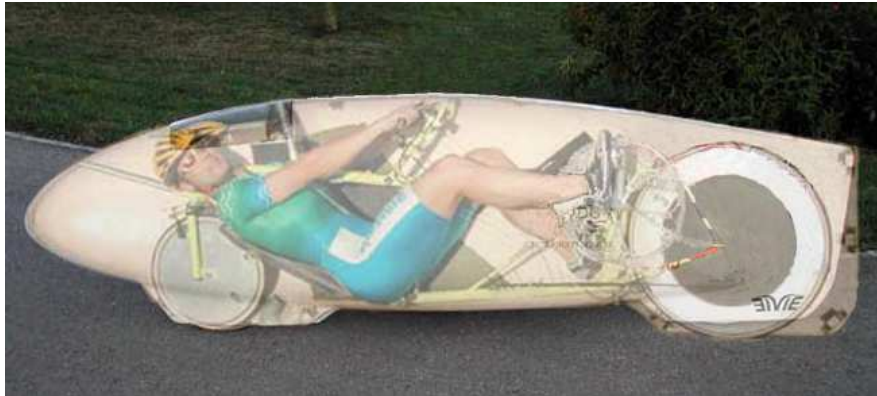
Figure 4.2: A bicycle propelled by a person lying inside a completely closed fairing.
