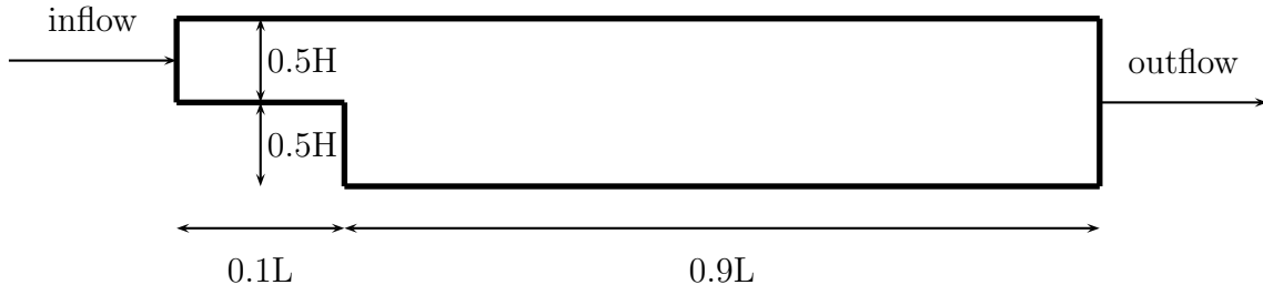
Figure 5.29: Geometry of the backward facing step problem. The H/L ratio is 15.
