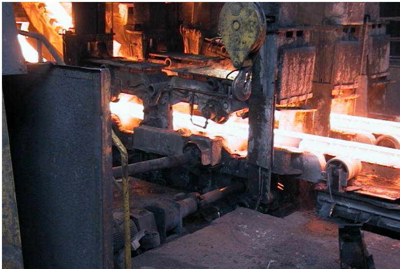
Figure 1.2: Casting machine for continuous casting of billets in the Štore Steel company.
