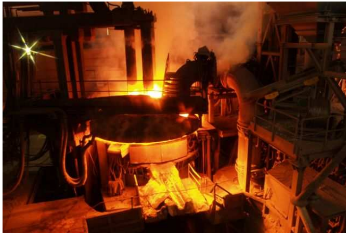
Figure 5.3: CC of steel: the ladle (Štore Steel company).
