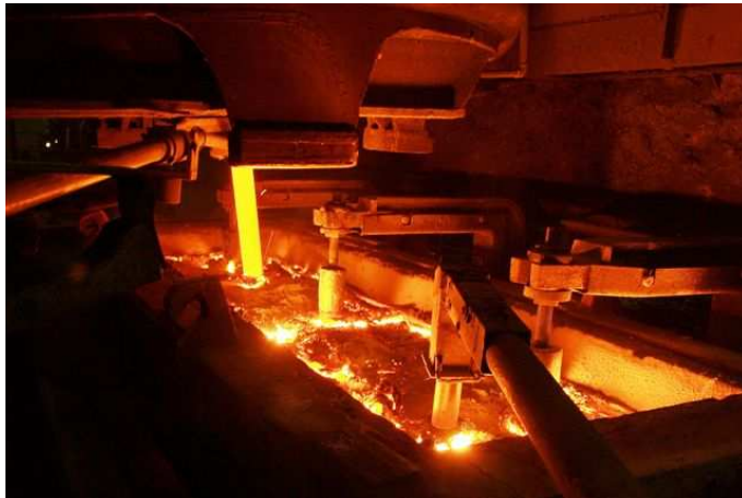
Figure 5.4: CC of steel: the tundish (Štore Steel company).
