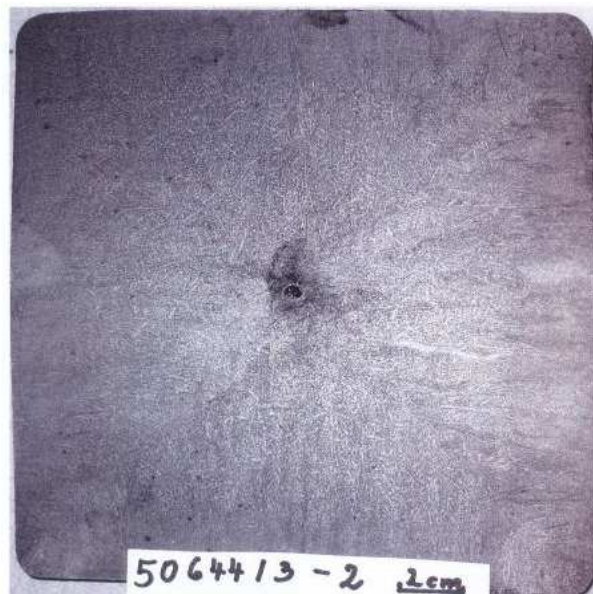
Figure A.18: Baumann print for steel 51CrV4, dimension 180 mm, without EMS.
