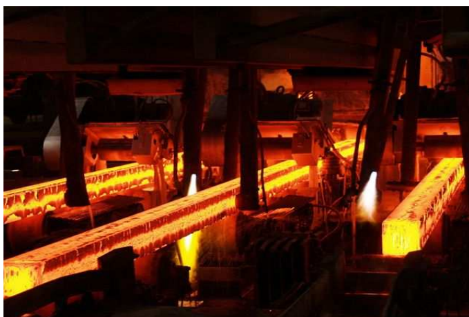
Figure 5.5: CC of steel: the billet (Štore Steel company).
