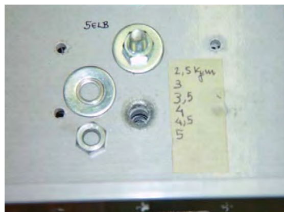
Figure 5.54. View after application of 50 Nm (equal to 31250 N) on bolt
