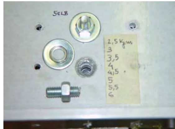
Figure 5.56. View after application of 60 Nm (equal to 37500 N) on bolt
