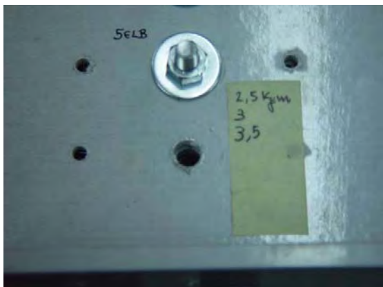
Figure 5.51. View after application of 35 Nm (equal to 21875 N) on bolt
