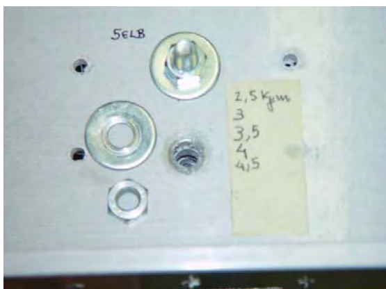
Figure 5.53. View after application of 45 Nm (equal to 28125 N) on bolt
