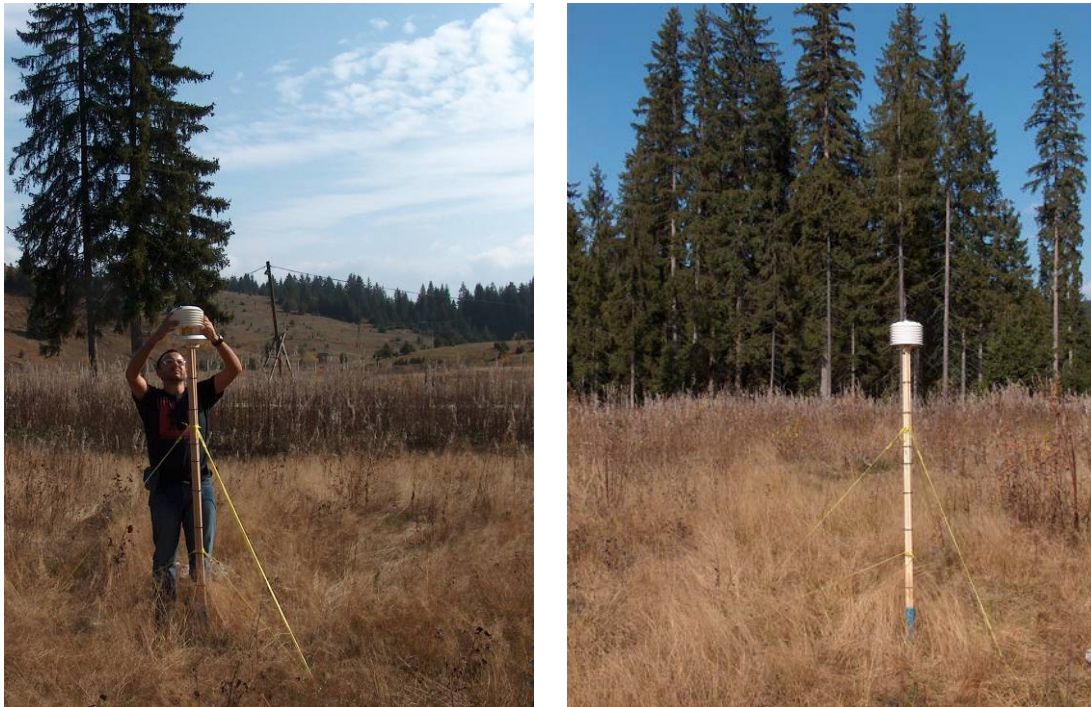
Figure 3-2: Mounting of the external temperature data logger. For location refer to Figure 3-8.
