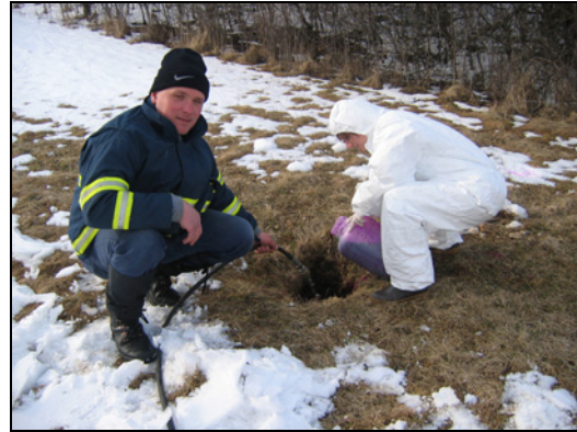
Figure 9.20: Injection of a tracer into an estavelle of the Šembijško Jezero (photo: A. Delost).
