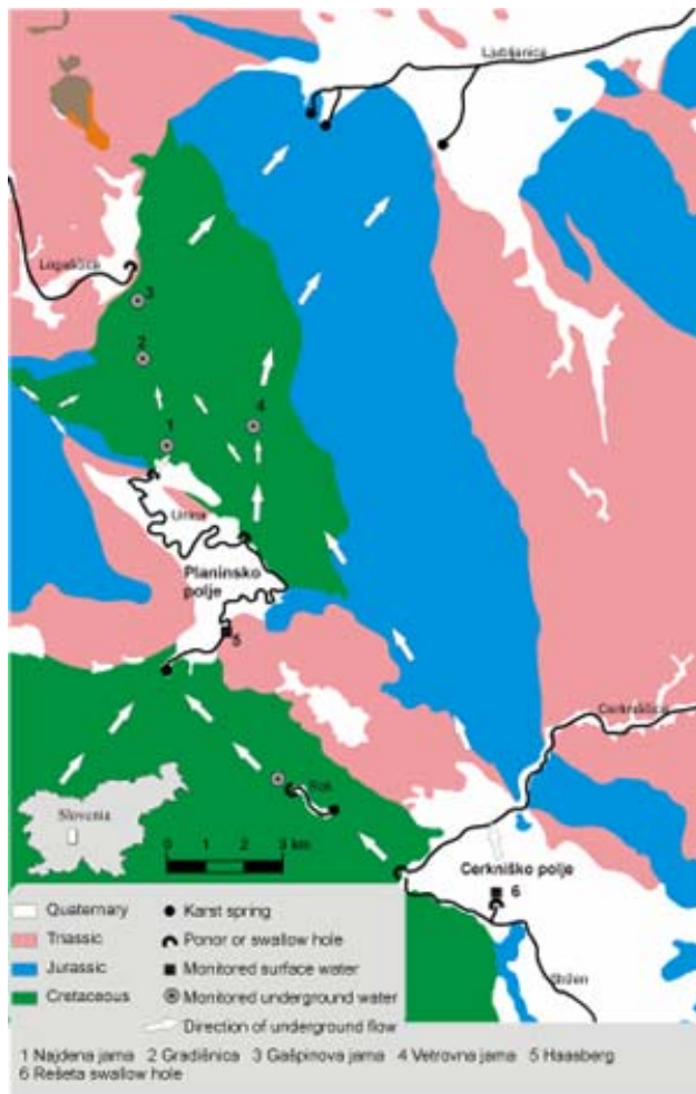
Figure 7.1: Geological map of studied area with measuring stations. The arrows indicate supposed underground flow.
