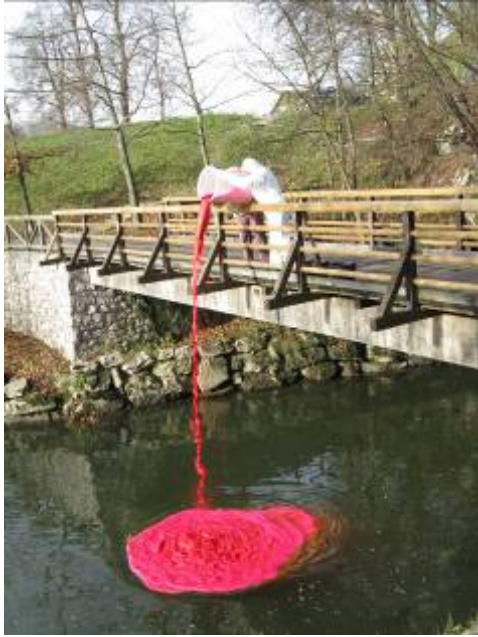
Figure 6.79: Solution of Sulphorhodamine G was injected into the Pivka River from the bridge just front of the ponor (photo: J. Turk).
