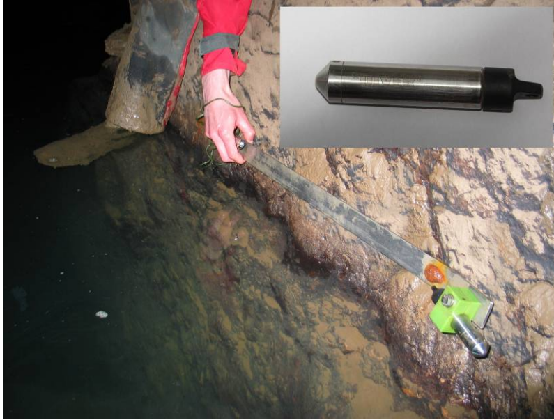
Figure 2: Data logger, which we used to measure level and temperature of underground water in caves (Photo: F. Gabrovšek).
