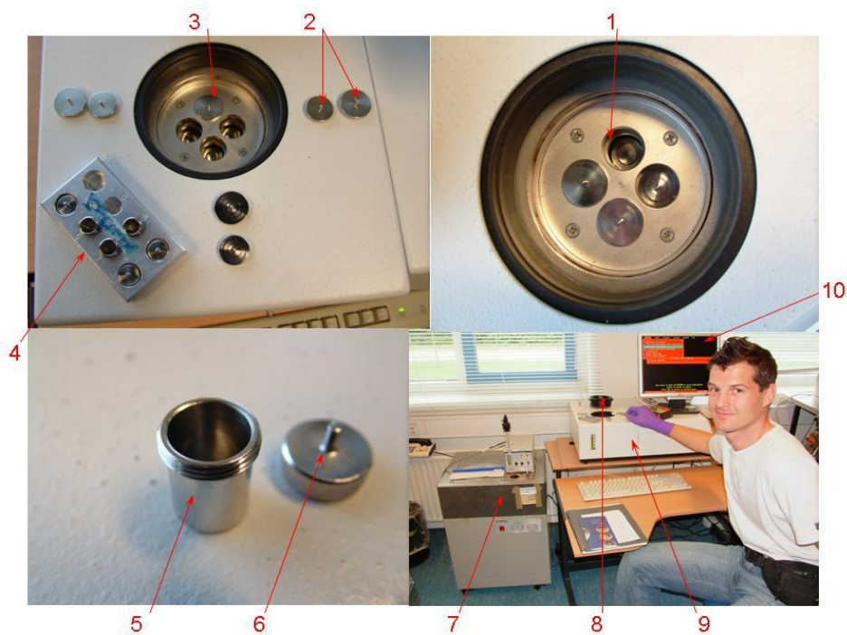
Figure 14: Microcalorimeter MC-DSC (Calorimetry Science Corp., Lindon, UT). 1 – one of four isolated calorimeter chambers , 2 – two lids for cover chamber, 3 – reference chamber, 4 – holder for containers and first lids, 5 – steel container, 6 – first threaded lid with a gasket, 7 – tempering pool with antifreeze solution, 8 – last cover lid for all four chambers, 9 – calorimeter
