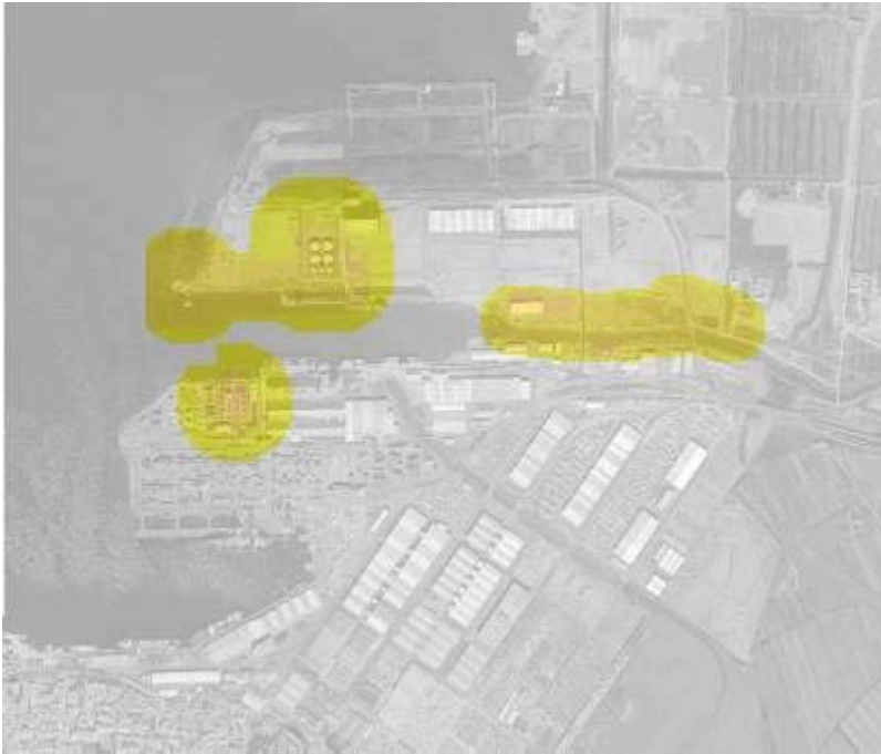
Figure 6: Threat index map for thermal radiation for the Port of Koper
