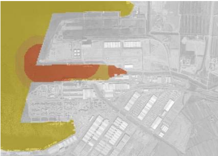
Figure 8: Threat index map for toxic release into the water from the liquid cargo (chemicals) terminal
