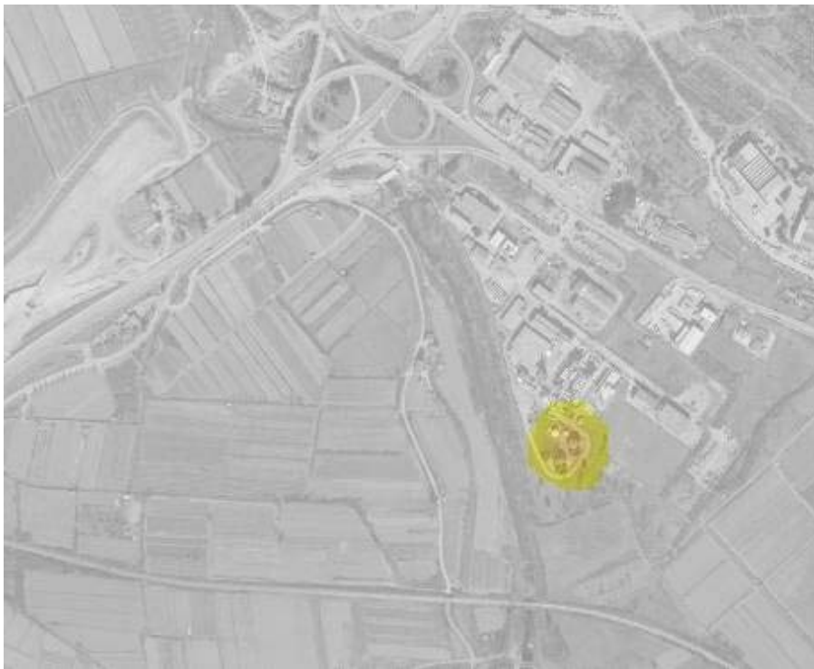
Figure 15: Threat index map for toxic release of o-xylene fumes at the R1 and R2 reservoir area into the air
