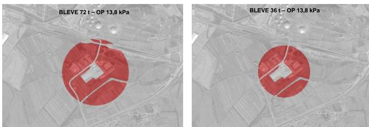
Figure 22: Impact area for BLEVE scenario for overpressure (OP) 13,8 kPa based on the sensitivity analysis of the quantity of LPG exploded
