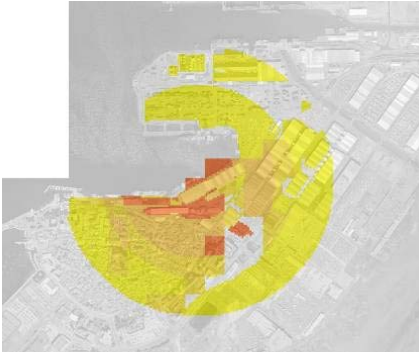
Figure 7: Threat index map for toxic release (ammonia) into the air from the fruit terminal
