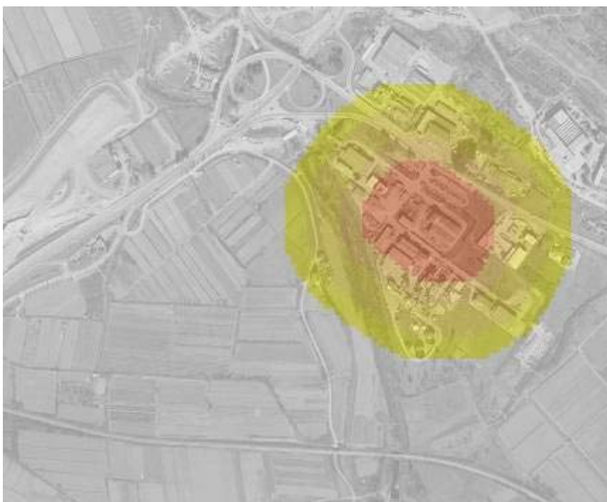
Figure 17: Threat index map for the release of vinyl acetate and butyl-acrylate into the air
