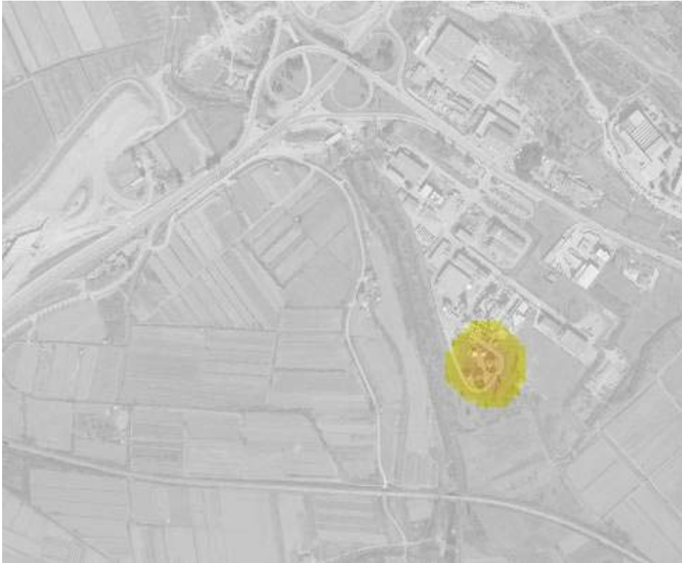
Figure 14: Threat index map for thermal radiation – the ignition of o-xylene fumes at the R1 and R2 reservoir area
