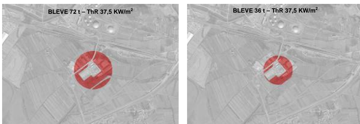
Figure 21: Impact area for BLEVE scenario for thermal radiation (ThR) 37,5 KW/m 2
