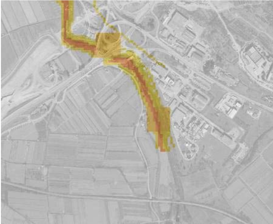
Figure 16: Threat index map for toxic release into the water - o-xylene mixed fire-extinguishing water
