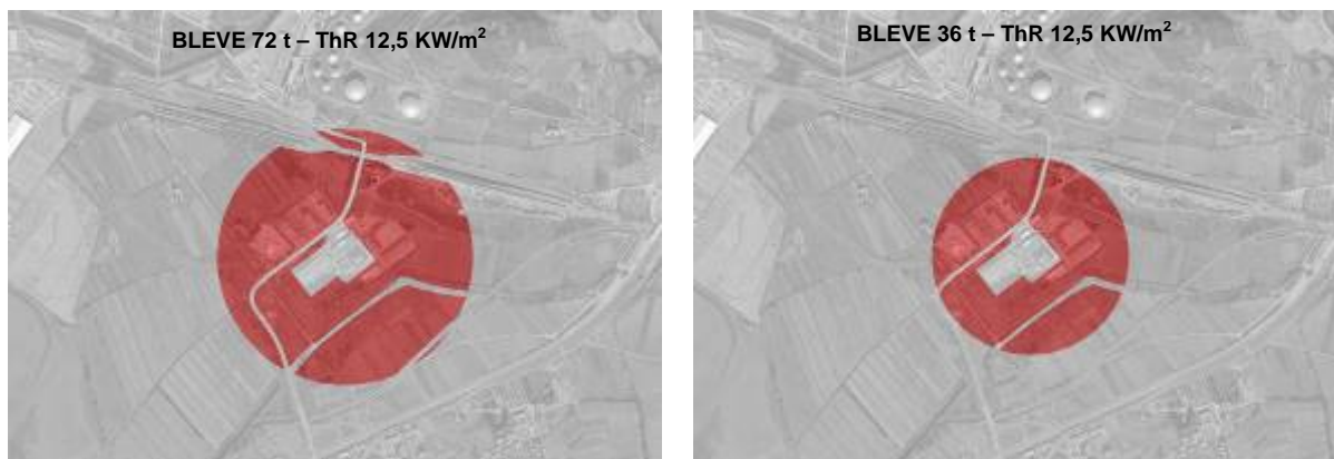
Figure 20: Impact area for BLEVE scenario for thermal radiation (ThR) 12,5 KW/m 2
