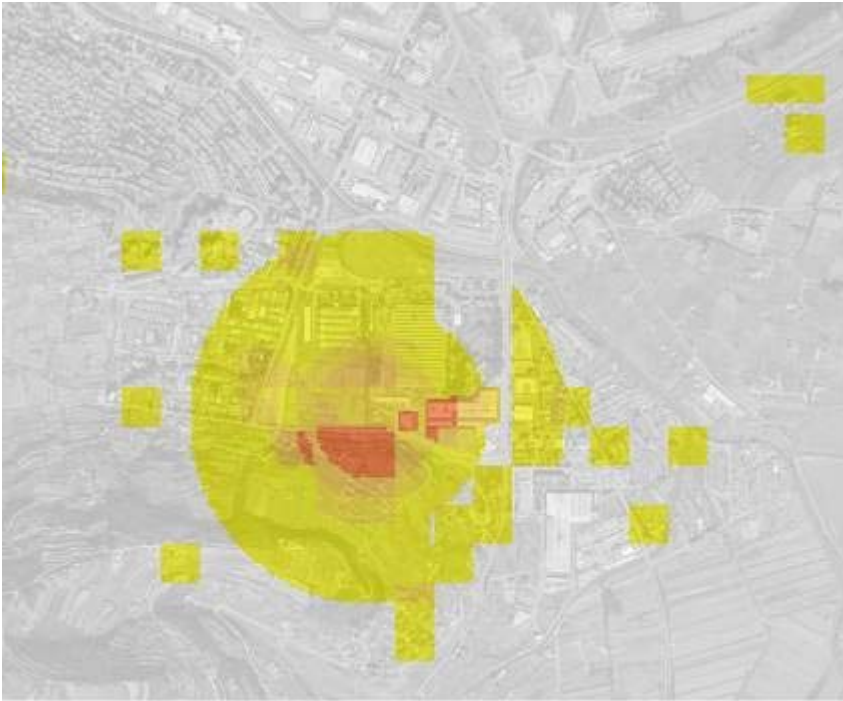
Figure 3: Threat index map for thermal radiation for BLEVE scenario
