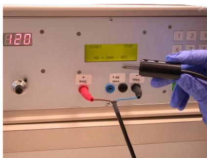
Figure 9: Electroporator and flat parallel electrodes used for electrotransfection
