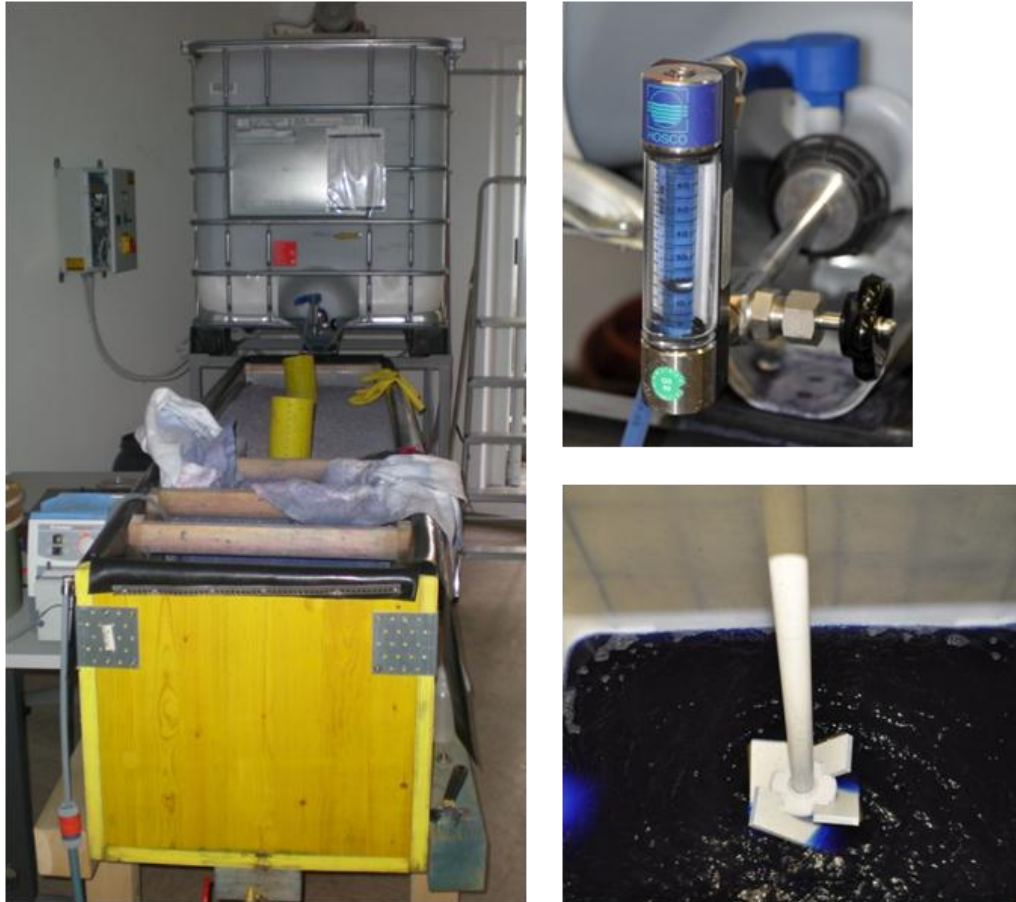
Figure 24: Photo of the CW model with reservoir, reductive stirrer and measuring valve.
