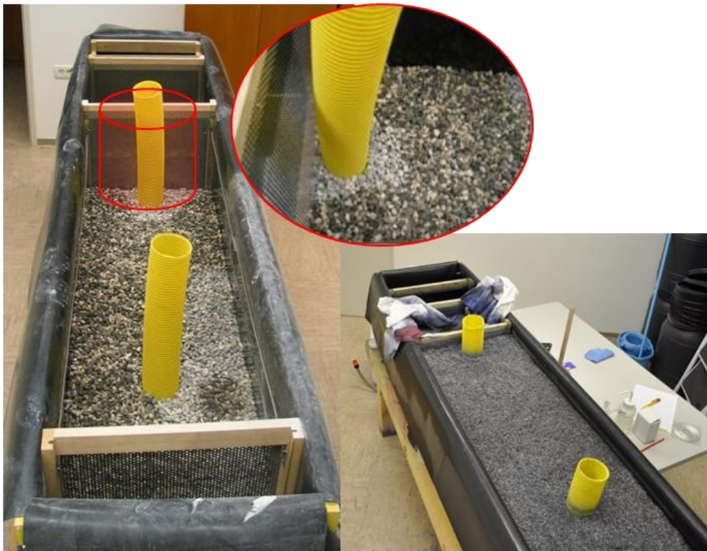
Figure 26: Photo of the media filled compartment, close look of the vertical sampling hose.
