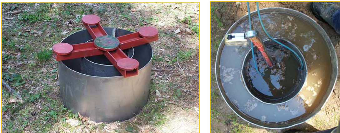
Figure 16: Set-up of double ring measurements
