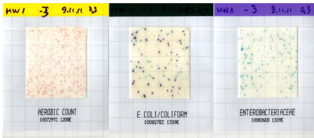
Figure 13: RIDA®COUNT plates, example of samples of wastewater from Postojna wastewater treatment plant, after 24 h of incubation at 35°C: left- RIDA®COUNT Total Aerobic Count; middle-RIDA®COUNT E. coli /Coliform; right- RIDA®COUNT Enterobacteriaceae.
