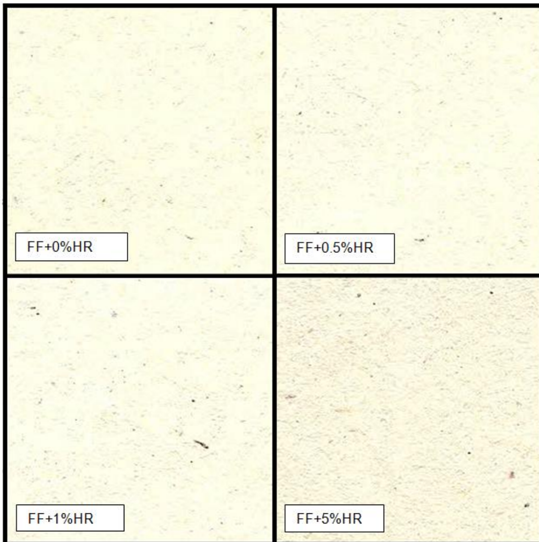
Figure 30. Formation of the middle layer of the cardboard with and without 0.5, 1 and 5% addition of SPH-WAS (HR), mixed with fresh fibres (FF).
