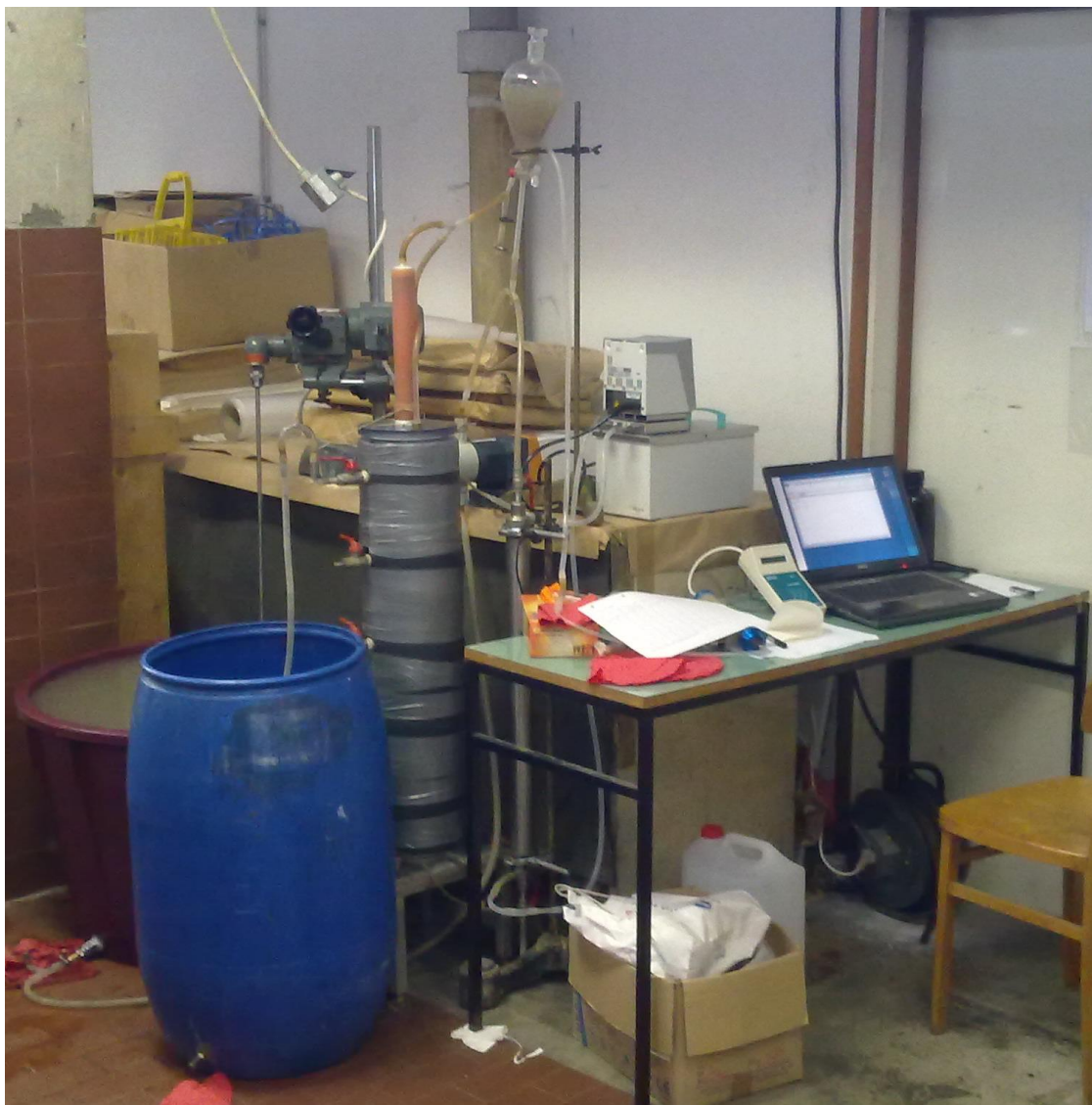
Figure 11. Pilot UASB reactor.
