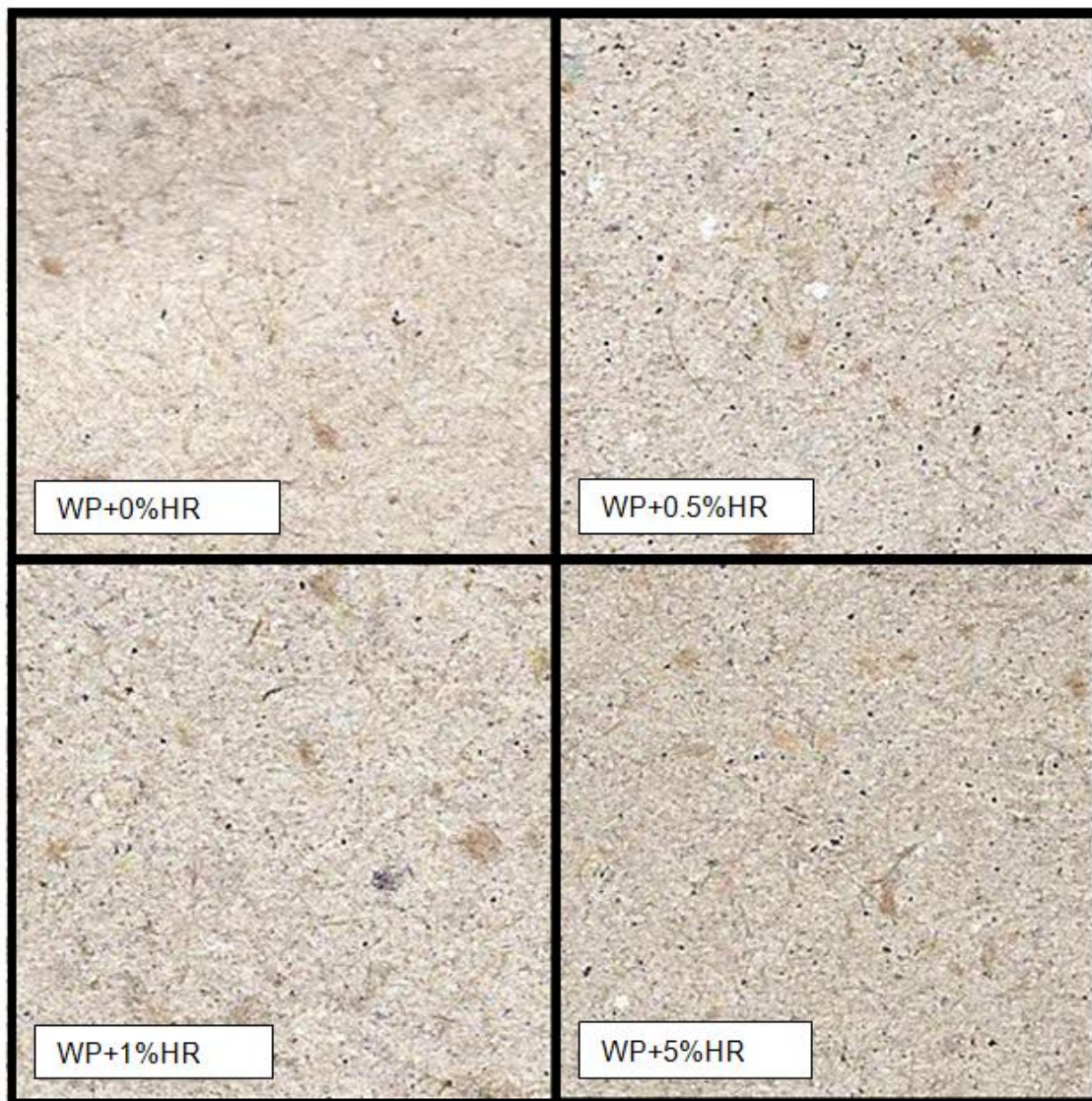
Figure 31. Formation of the middle layer of the cardboard with and without 0.5, 1 and 5% addition of SPH-WAS (HR), mixed with waste paper fibres (WP).
