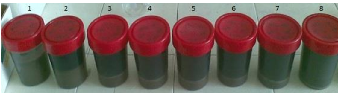
Figure 19. Settling (1 hour at 4 °C) of particles in a series of hydrolysed samples at pH 12 and 95 °C. The first (1) is the original WAS, followed by samples hydrolysed for different times up to 24 hours (2-8): 0, 1, 2, 3, 4, 18 and 24 hours.
