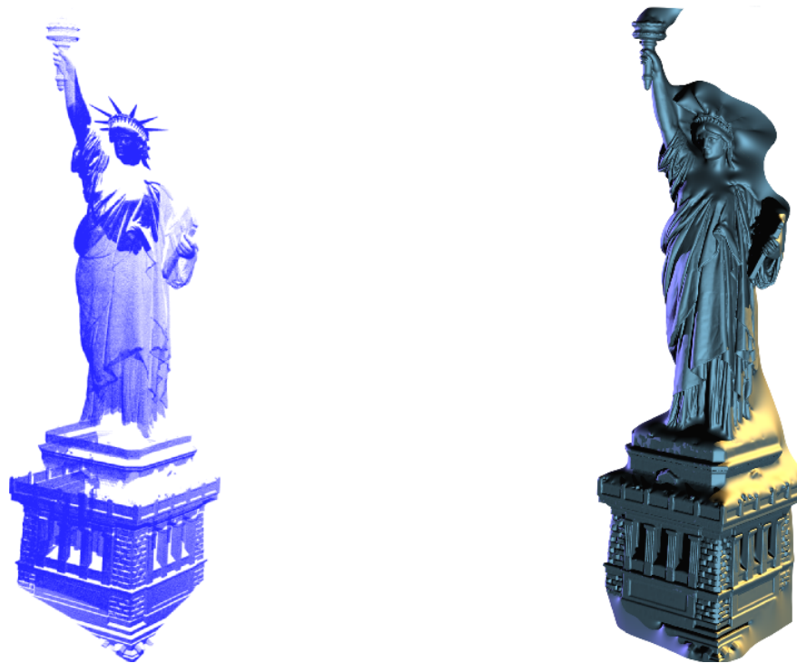
Figure 3.5: Surface fitting problem. Left picture - raw point-cloud from a LIDAR scan of the Statue of Liberty, right picture - surface, reconstructed by the RBF interpolation. The few viewpoints, oblique scanning angles and large gaps make this a difficult problem for other techniques [Carr et al. , 2003].
