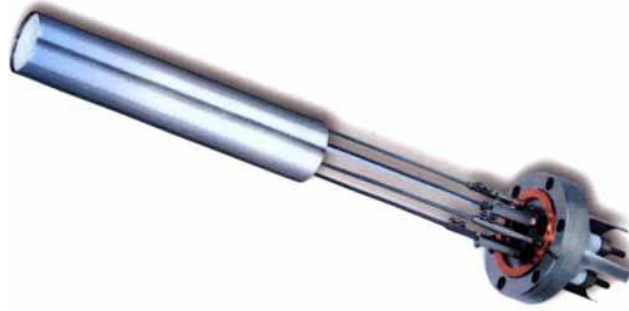
Figure 3.2: Photograph of a low temperature Knudsen evaporation cell. The organic material and heating element are located within the stainless steel cylinder connected to the mounting element by thin metallic rods for low heat transfer.
