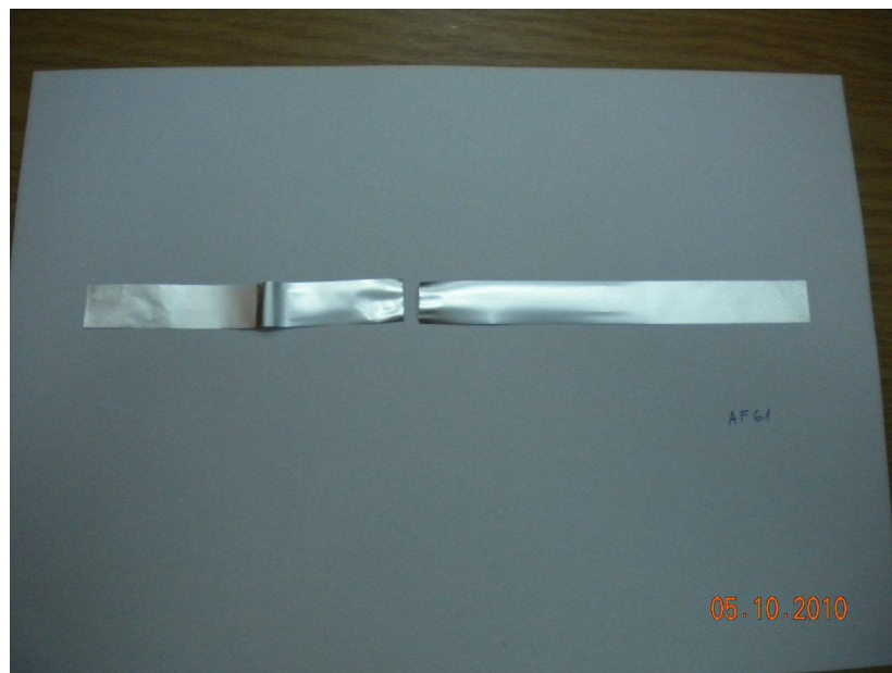
Figure 4.5: Sample after tensile strength and elongation testing (Photo author, courtesy Impol)
