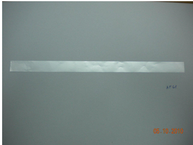
Figure 4.1: Sample before tensile strength and elongation testing (Photo author, courtesy Impol)
