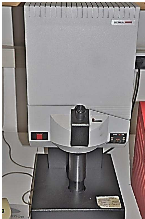
Figure 20: Equipment (Datacolor Spectraflash SF 600 PLUS) for measuring CIEL*a*b* colour differences.
