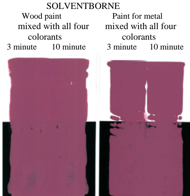
Figure 38: Colour shade on solventborne products; wetting and compatibility test.
