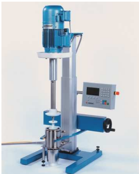
Figure 26: Rubbing machine for the paint pastes [37].
