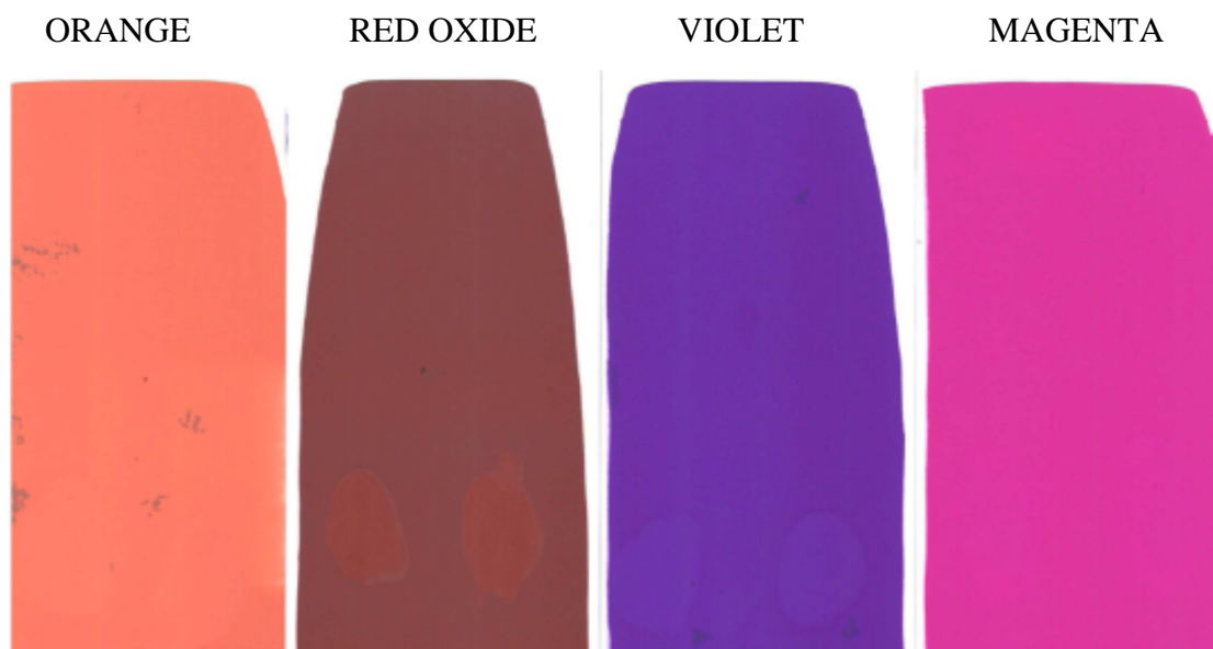
Figure 37: Solventborne paint for metal (enamel) and our samples universal colorants (compatibility test, rub-out test).
