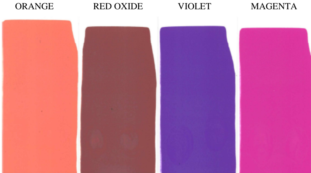
Figure 35: Solventborne wood paint and our samples universal colorants (rub-out test).
