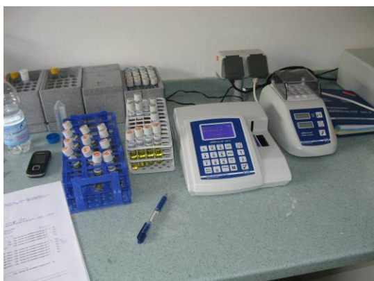
Figure 4.8: NH 4 + determination with Nanoclor 500 D photometer
