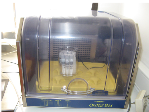
Figure 4.6: The incubation of the samples for BOD 5 determination
