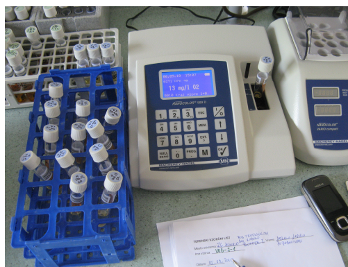
Figure 4.7: BOD 5 determination with Nanoclor 500 D photometer
