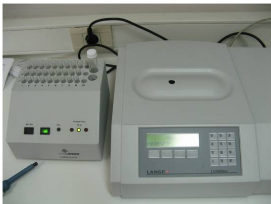
Figure 4.10: Determination of toxicity with the luminescent bacteria test ( Vibrio fischeri ) using the LUMISTox-300 luminometer and LUMISTherm incubator
