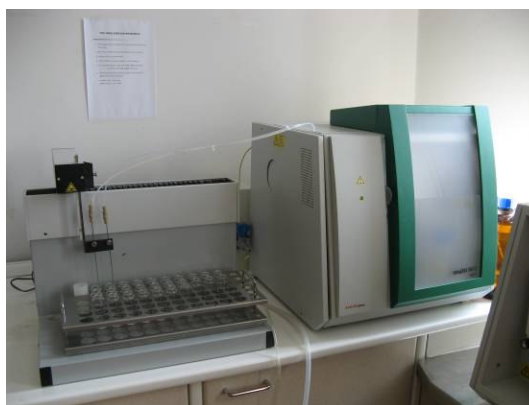
Figure 4.9: Determination of TOC concentration with Analytic Jena Multi C/N 3100 analyzer
