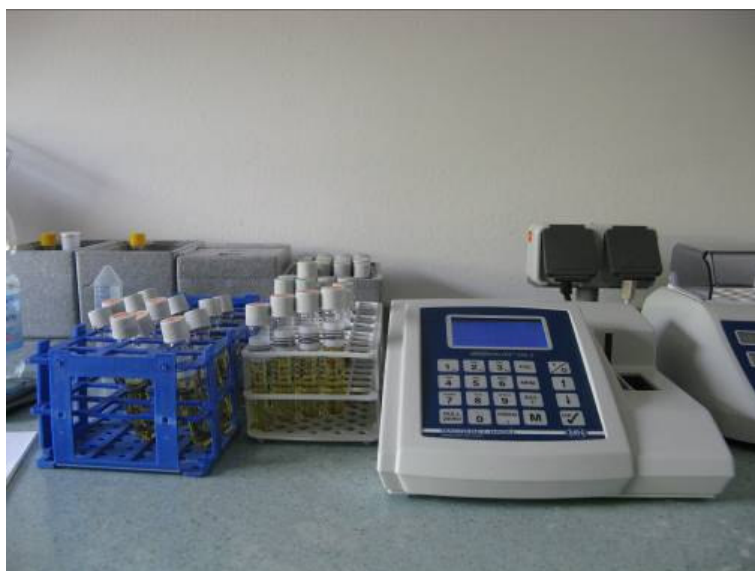
Figure 4.5: COD determination with Nanoclor 500 D photometer
