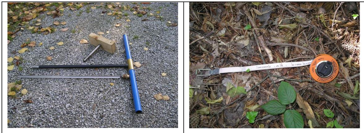
*Figure 18: Steel increment borer used for sampling (left) and girth measuring tape (right) (photo: J. Lah)*
