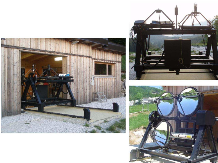
Figure 3.2: LIDAR system: LIDAR sliding on rails from inside the shelter (left); vertical and horizontal LIDAR positions (right top and bottom).
