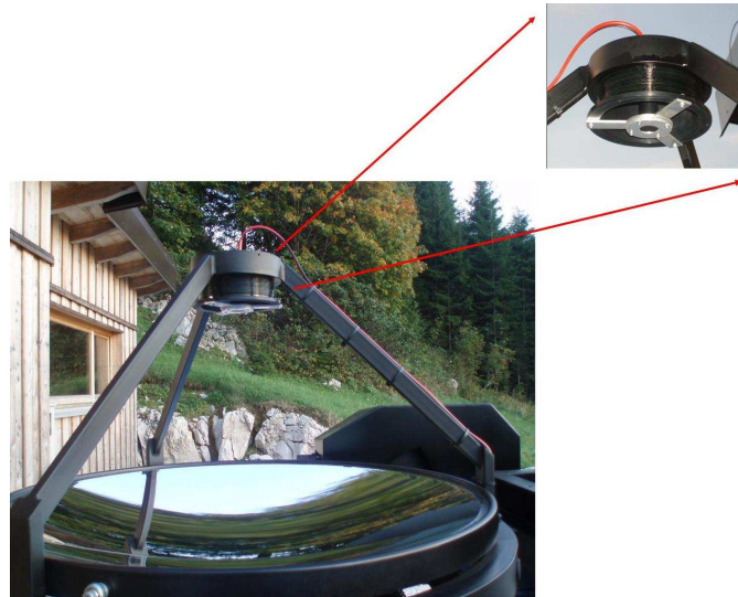
Figure 3.4: Receiver and detector of the LIDAR system at Otlica: the parabolic mirror and photo-multiplier. The PMT is placed on the focal point of the mirror.
