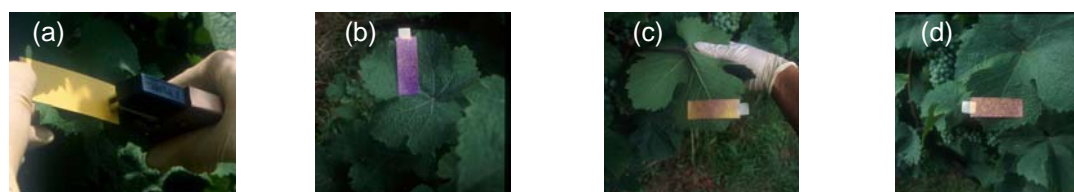
Figure 7.9: Location of WSP on vine leaves: (a) stapling WSP on vine leaf, (b) position of WSP on vine leaf after application, (c) WSP on lower leaf side after application, (d) WSP on upper leaf side after application (Photo: Simona Luskar).
