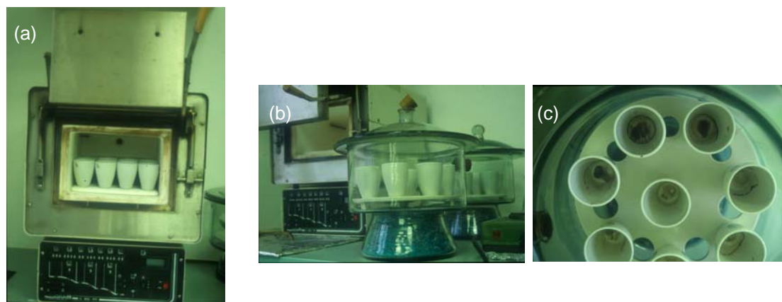
Figure 7.8: Processing during dry ashing of filter papers: (a) porcelain crucibles with filter paper strips in kiln before ashing, (b) cooling porcelain crucibles, (c) ash of filter paper strips in crucibles (Photo: Simona Luskar).
