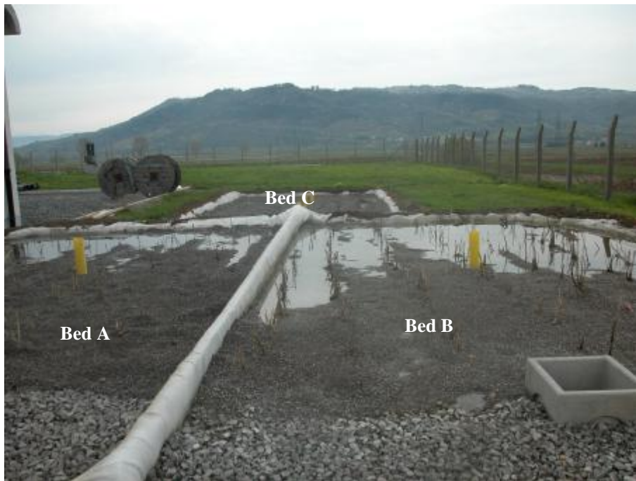
Figure 12: Wetland pilot plant planted in April with young plants of Phragmites australis . Source- photo Lucija Kobal, 2004.
