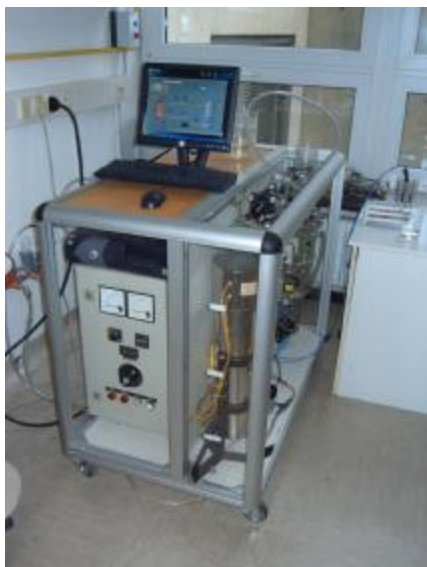
Figure 17: Photo and schematic of Solvay Interlox pilot plant; P = pump, UV= UV reactor, R = reservoir with waste water, H 2 O 2 30%=hydrogen peroxide with 30% concentration, V= sample draw. Source- Majcen-Le Marechal, 1997.
