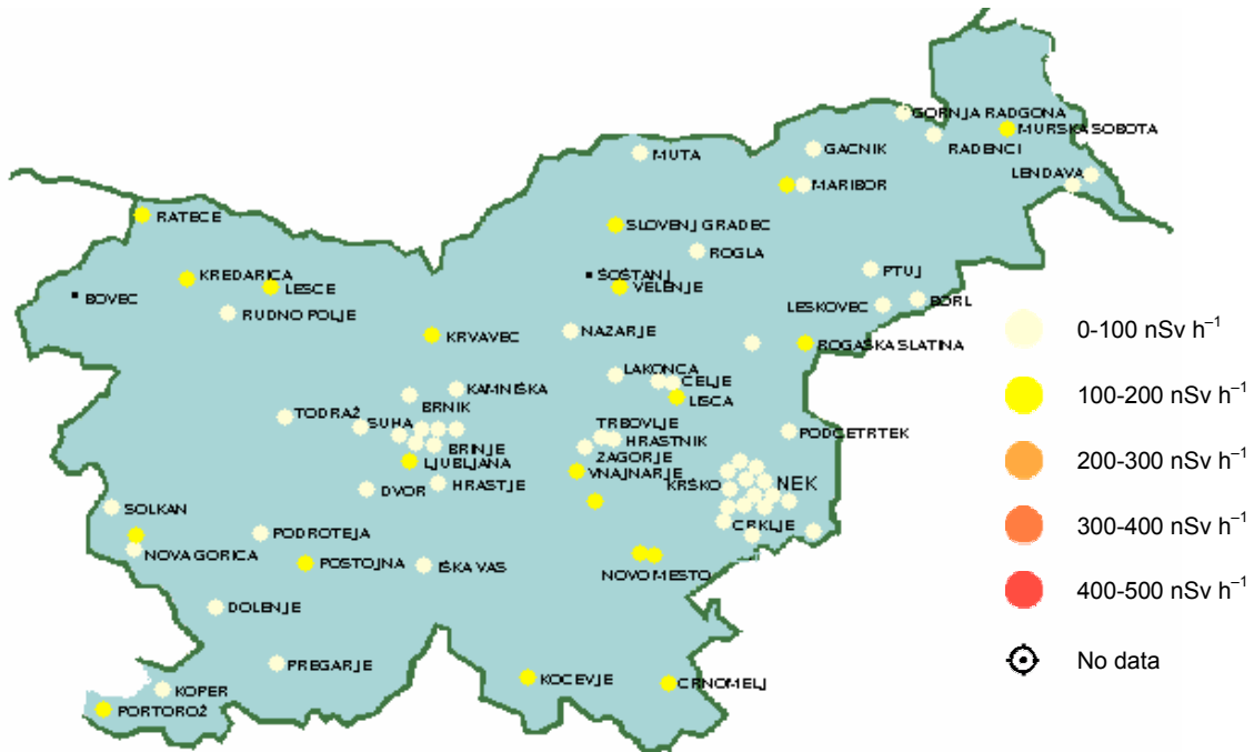
Figure 4.4: Map of Slovenia with measurement locations for external radiation (External gamma radiation, 2007).
