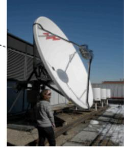
MIDAS/AMBER: use a parabolic dish reflector instrumented with an array of feeds, 'Radio fluorescence'.
