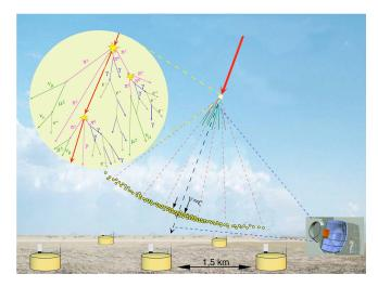
• Extensive air-showers (EAS) induced by collisions of primary cosmic particles with atoms of the Earth's atmosphere
