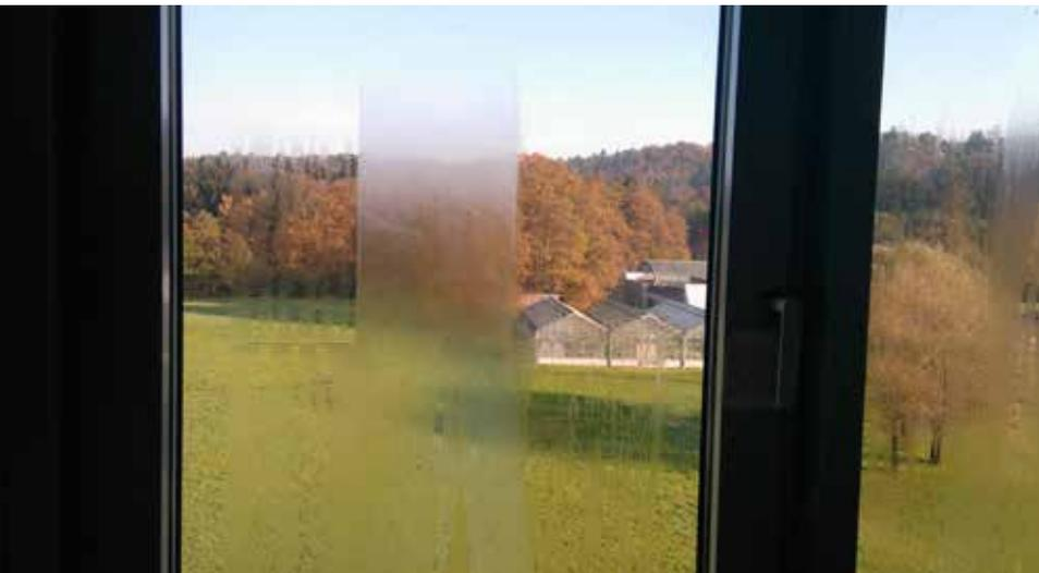
Antifogging thin film on window: less active left, more active right, no coating in the middle.
