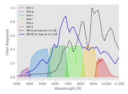
**Figure 2.** The filter response system that will be on the Rubin Observatory overplotted with a typical spectra of SN Ia and SN IIP. The redshift of the SN spectra is at 1.28, as the examples from Figure 3 where multiply-imaged galaxies in Abell 370 are shown at which the survey will be sensitive, considering the image depth and the magnification from the galaxy cluster.
